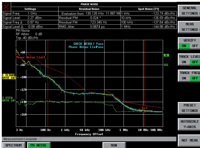
Phase noise measurement with the R&S®FS-K40 application firmware.
